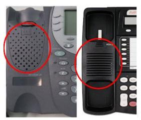
If your phones speaker is not directly under the phones receiver then you will need to detach the ring detector that is stuck under the lifter - this just pops off and then re stick it over the phones speaker.
