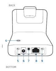
Step 3 – The cable that comes in the box with the headset – needs to be plugged into the back of the Plantronics headset base (port 8 on the above diagram) and then into
