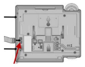
Step 2 – using the cable with the 2 pin connector ends rather than the square telephone plugs plug one end into the black box on the ehs and the other end into port 7 on the back of the Plantronics headset base as per below diagram.
