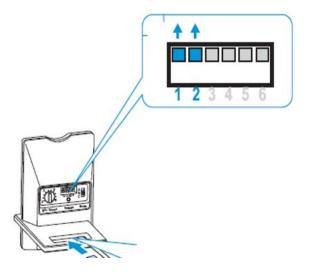
If you are using one of the Sennheiser SDW headsets you will need to make sure that the number 1 switch is all the way down, and number 2 all the way up.
