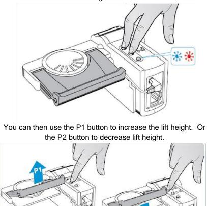
Once you are happy with the positioning you can hold the P1 and P2 buttons down again until the LED's stop flashing. This will save the height you have set.
