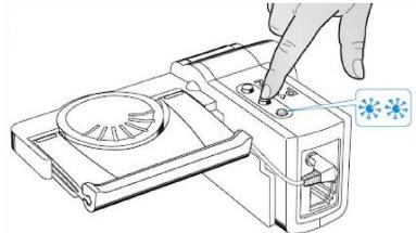
To Program the first ring tone we are going to press the P1 button until the LED flashes Blue. Then get someone to call your phone. Don't pick it up just let it ring. If the lifter has detected the ring tone the LED will flash red three times. If there is no flash then the lifter can not detect the sound. Refer to the next troubleshoot step to resolve this issue.
