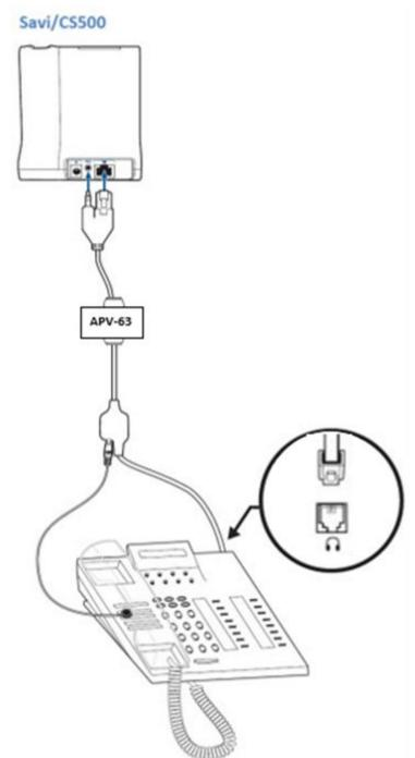
Looking at your EHS cable, the larger of the plugs (combination of an RJ and pin connector) will plug into the base of your headset.
