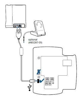
The APU-76 cable converts previously desk phone only headsets into USB headsets, alternatively it also provides EHS connection for phones with USB headset ports.
