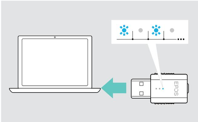
The dongle controls the wireless communication between computer and headset.
