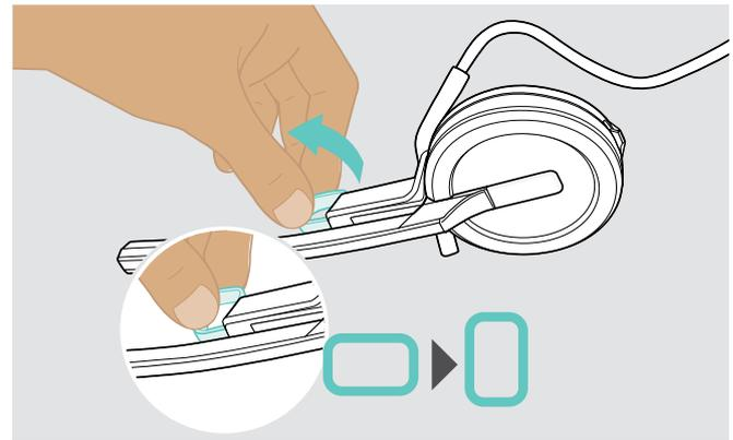
▷ Rotate the cheek spacer to increase or decrease the distance between the microphone and your mouth – if required.
