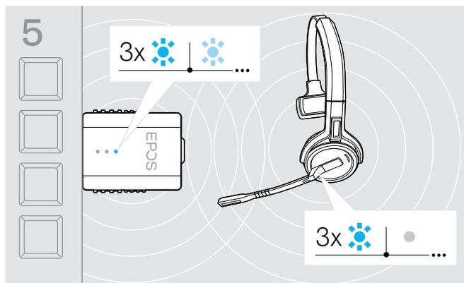
If pairing is successful, the dongle LED lights up dimmed blue and the headset LED switches off.
