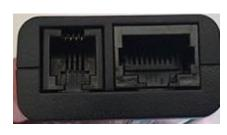
Plug 3 of the Jabra Y cord plugs into the port on the right on the EHS 40 box (the bigger of the 2 ports).
