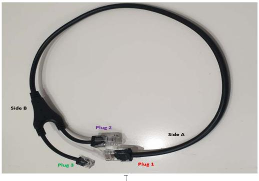
The Sennheiser Y cable has 3 connections total. The 2 cables on side B are split in a Y than the cable opposed to Side A which is one connection.
