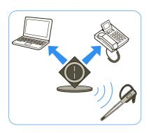
You can use the headset system with your fixed line phone (Phone mode) and/or your PC (PC mode). The base station controls the wireless communication between the products.
